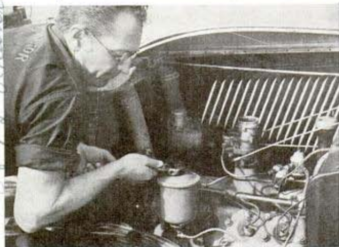
Now that good oil filters are available, engine oil can be used for long periods without draining the crankcase. However, watch oil condition and replace filter periodically
